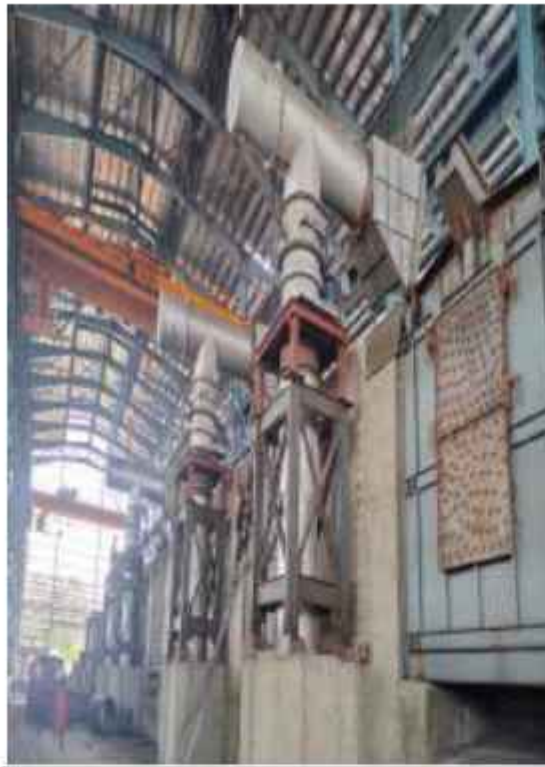
Bag Filter for Steel Smelting Shop
